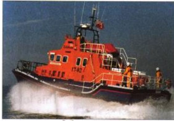
This Severn Class lifeboat is an all-weather lifeboat. It is the largest lifeboat at 17 metres long.
